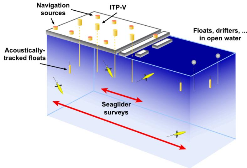
***Figure 1. Proposed experimental layout showing navigation sources, ice-tethered profilers, floats and Seagliders. Source spacing is approximately 100 km, and thus 8 sources cover at least 60,000 square km. (Courtesy Lee and Rainville, APL-UW).***
