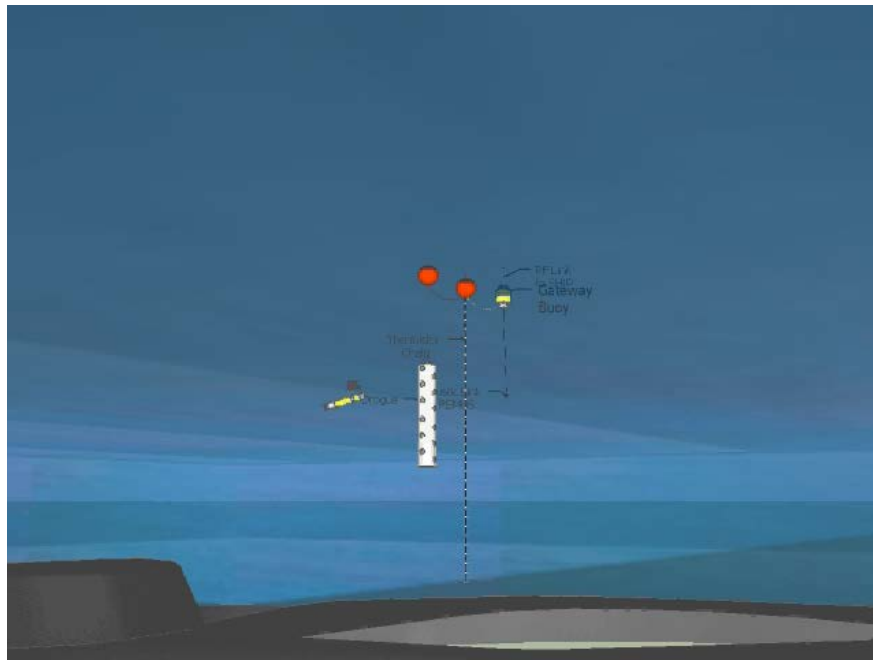
Figure 3 Three buoy drogue Gateway Communication system used in LatMix 2011. The leader buoy has a 10 m holey-sock drogue centered at 10 m depth. The second buoy contains a 16 element thermistor chain spanning 1m to 49 m. The third buoy is the hydroid Gateway communication buoy.
