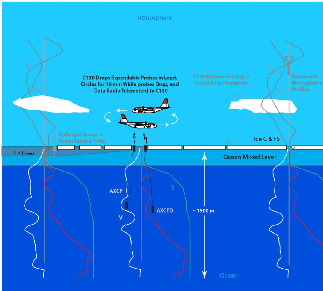
**Figure 1. Schematic of the SIZRS ocean column AXCTD & AXCP profiles. Stations will be made in five locations across the SIZ (3 shown) with at least one each in open water, MIZ, and pack ice. Buoys will provide upper ocean time series at several locations. The aircraft remote sensing will measure ice & cloud properties.**
