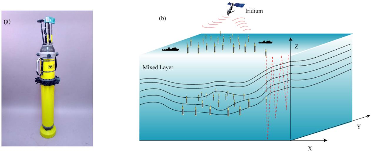
**Fig. 1: (a) EM-APEX float with dual  $\chi$  sensors. (b) Schematic of a spatial array of 10-microstructure EM-APEX floats ( $\chi$ -EM-APEX floats) and 10 regular EM-APEX floats. N.B. The  $\chi$  sensors were mounted so as to be out of the wake produced by the Iridium antenna, which will be tilted to the side in the so-called “Mai Tai” mounting.**
