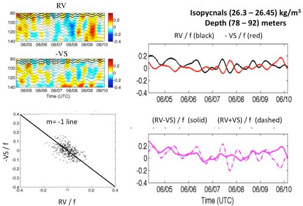
**Fig. 5: RV and VS at Site 1 between isopycnals 26.3 and 26.45 kg m<sup>-3</sup>. The compensating behavior of VS and RS indicates that much of the variability is caused by internal waves. However, there is a PV trend to the background linear PV in the early portion of the record.**
