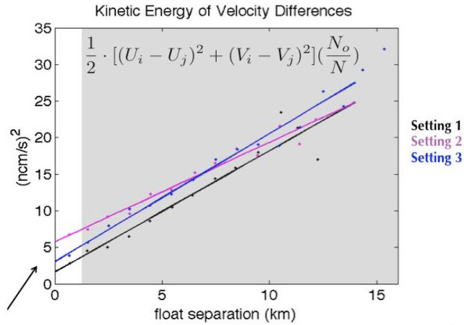
**Fig. 2: Velocity structure function, the square of WKB adjusted velocity differences vs. profiler separation, with all floats for the three settings. Intercept (arrow in figure) corresponds to 1-2 cm/s uncertainty.**
