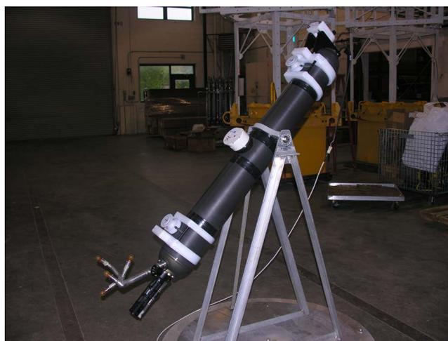
***Figure 3. Photograph of an ITP-V in the jig during a test spin to quantify sensor relative orientations. (Actual spin tests are conducted outside in an area free from artificial magnetic fields.)***
