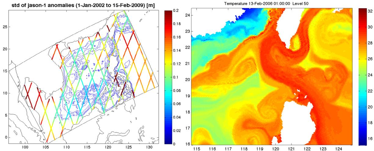
**Figure 1.** *Left: South China Sea ROMS model domain and the pattern of Jason altimeter ground-tracks. Color indicates sea level variance. Right: Example of surface temperature in the environs of the Luzon Strait revealing mesoscale to submesoscale variability.*
