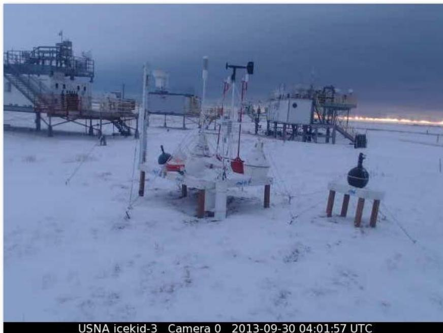
*Figure 4: Near real time webcam image from IK3T at the AOX site in Barrow, AK. 10 different Arctic drifters and other temperature sensors are co-located to determine if there is any bias between instruments. The IK3T has a meteorological package as well as webcams that will identify any snow accumulation or freezing up of instruments.*
