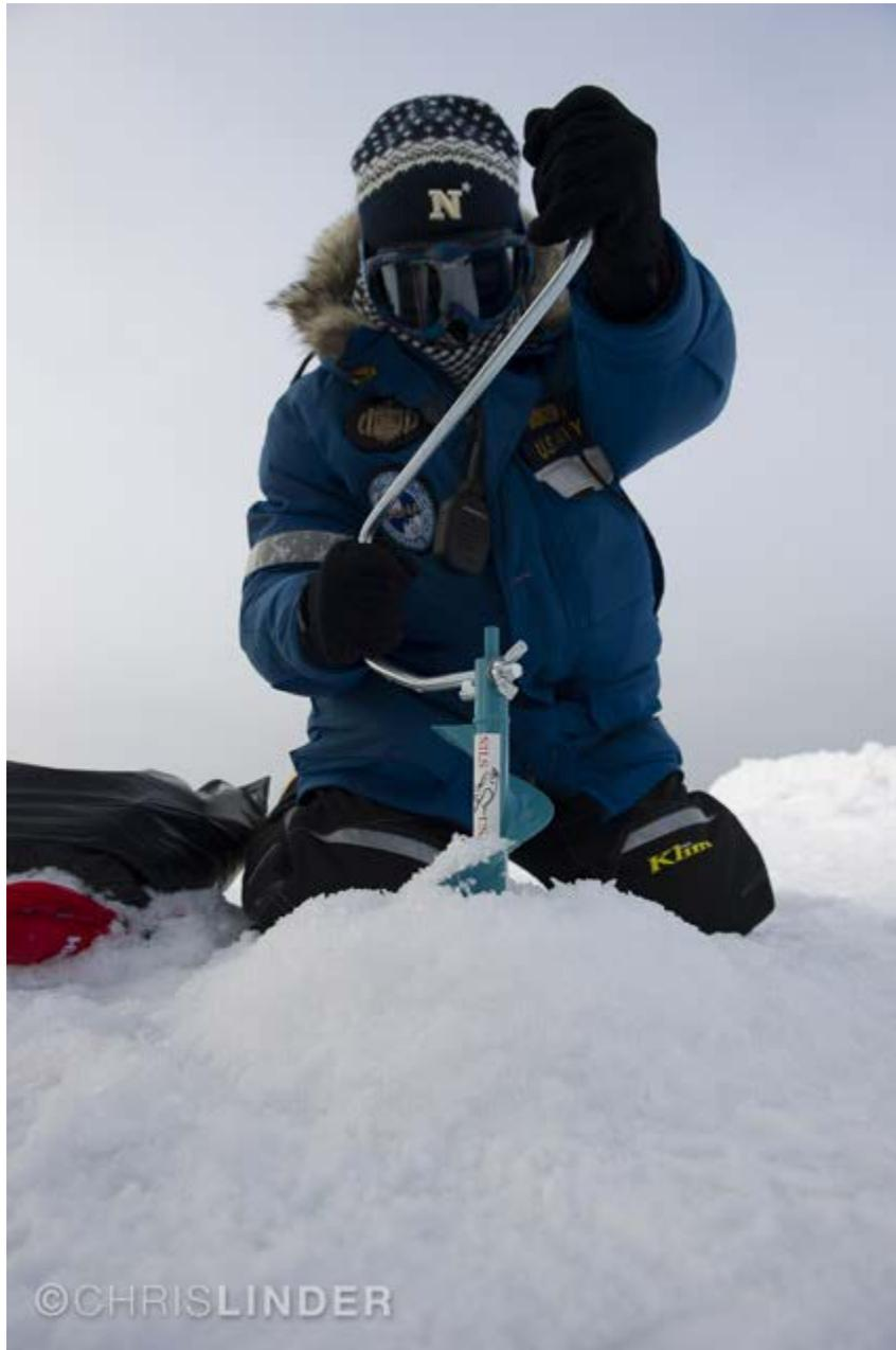
*Figure 2: The NAICEX field site just offshore Barrow, AK on the shore fast ice. USNA Midshipman drilling holes through the sea ice for thickness measurements. Over 40 holes were drilled along a 3 km survey line to better understand the under ice topography.*
