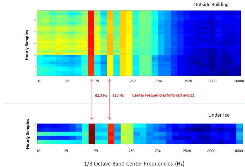
**Figure 6: Open air (top panel) and under ice (bottom panel) spectral signatures. Relative 1/3 octave noise levels are shown for the 30 hours of open air and 5 hours of under-ice sampling. Single spectral signatures were transmitted hourly via iridium modem. Data was downloaded from the sensor's internet site and post processed for visualization. A 60 Hz noise ground and its 120 Hz harmonic are clearly visible.**
