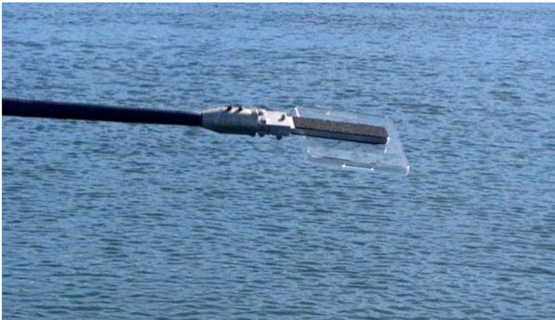
*Figure 2. "Plate" style samplers. Top, sterile laboratory-grade polystyrene plate with velcro patch attached to back; Bottom, view of plate attached to pole with velcro.*
