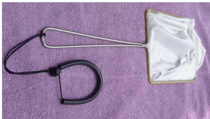
*Figure 1. Custom-designed stainless steel hoop nets used to maximize fecal sample collection weights from beaked whales.*
