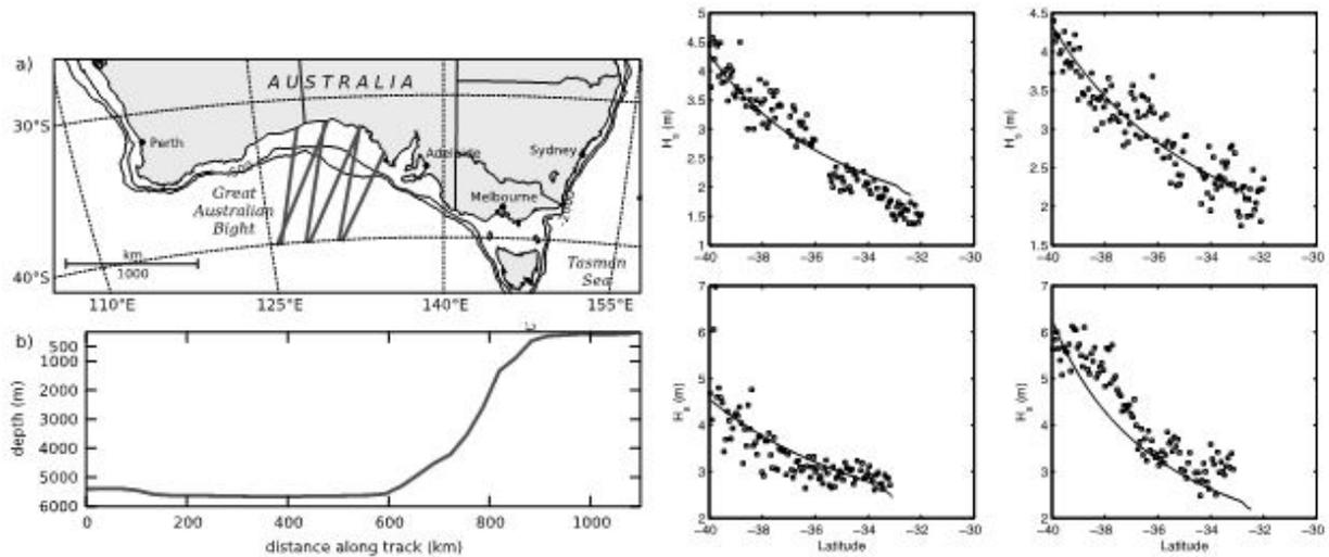
**Figure 1. Remote sensing study, used to calibrate the swell-dissipation term (Young et al., 2013a). (left) The study area in the Great Australian Bight region of the Southern Ocean with typical altimeter ground tracks (top); variation of water depth along a typical altimeter great circle path (bottom). (right) Four typical cases of the measured (altimeter) decay of the swell along the transects (squares). The predicted decay from the model is shown by the solid line.**
