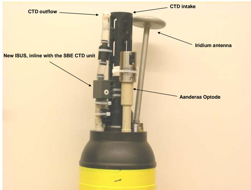
**FIGURE 2.** The upper endcap of a profiling float with the inline ISUS unit. A number of floats of this design have been deployed, both the research version produced by UW and MBARI and the commercial version produced by Teledyne/Webb and Satlantic.
