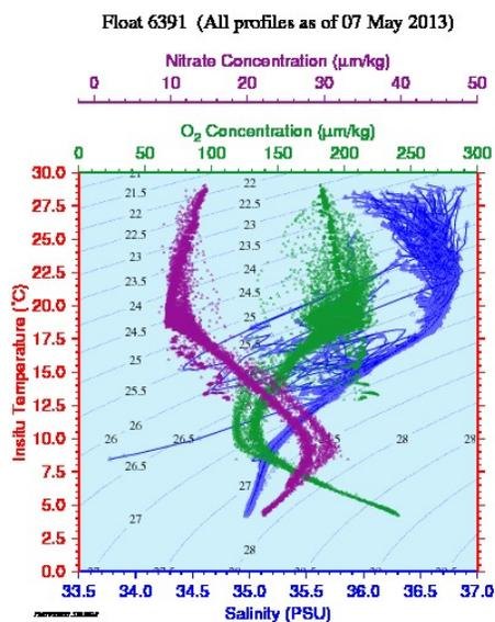
**FIGURE 4. Top panel: Temperature, salinity, dissolved oxygen, and nitrate data from 266 profiles from UW profiling float number 6391 in the North Atlantic near Bermuda. The profiles were collected at 5-day intervals between October 2009 and May 2013. Bottom panel: Salinity, dissolved oxygen, and nitrate plotted as functions of temperature from float 6391.**
