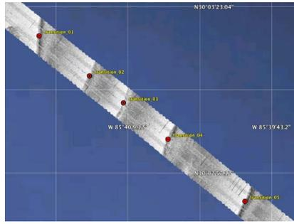
**Fig. 3. Map showing the main reverberation measurement track at TREX13, and the detected "transition" zones in which the texture of the sediment appeared to change. [Map of a part of the TREX13 test area showing the initial multibeam survey swath.]**
