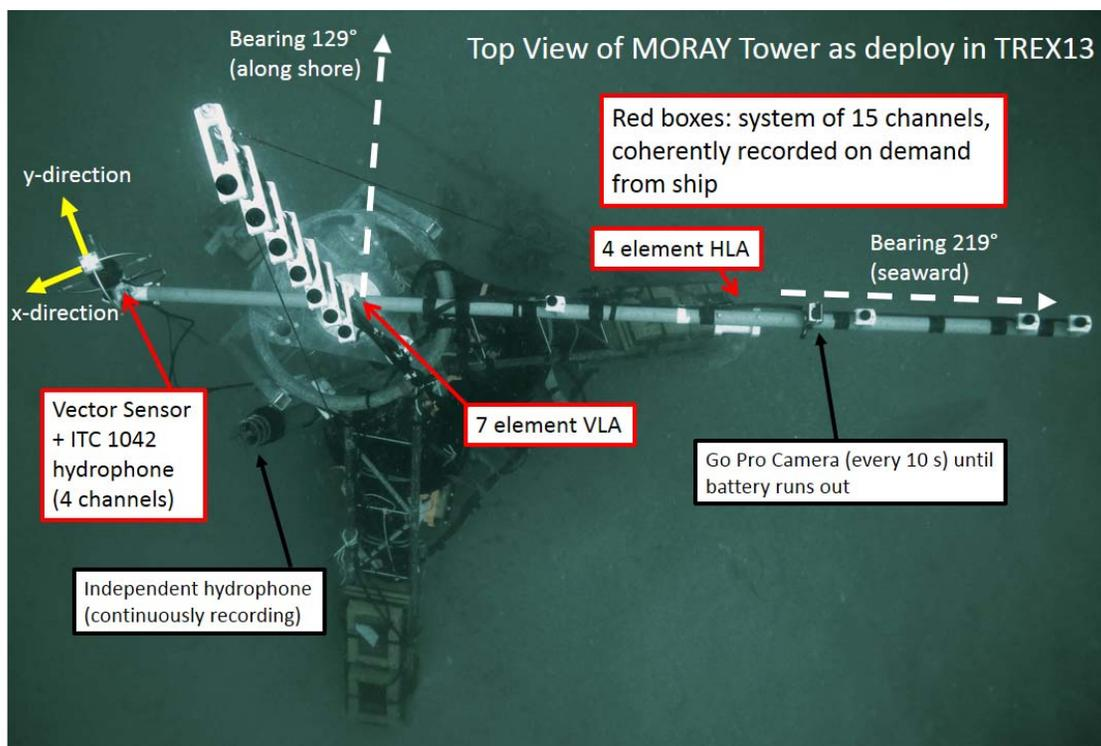
**Figure 3.** Dive photograph of the MORAY tower made just prior to its recovery from the TREN13 experiment, with its key elements identified. The neutrally buoyant VHS-100 vector sensor is shown on the left suspended within its framework.
