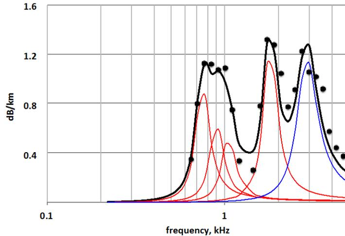
**Figure 3. Depth averaged values of attenuation coefficients,  $A$ , during the day and theoretical calculations for swim bladders with resonance frequencies of 0.75, 0.9 and 1.05 kHz hypothetically due to adult hake, 1.8 kHz hypothetically due to juvenile (2 year old) hake, 2.9 kHz due to an unknown species (blue), and the sum (in black).**
