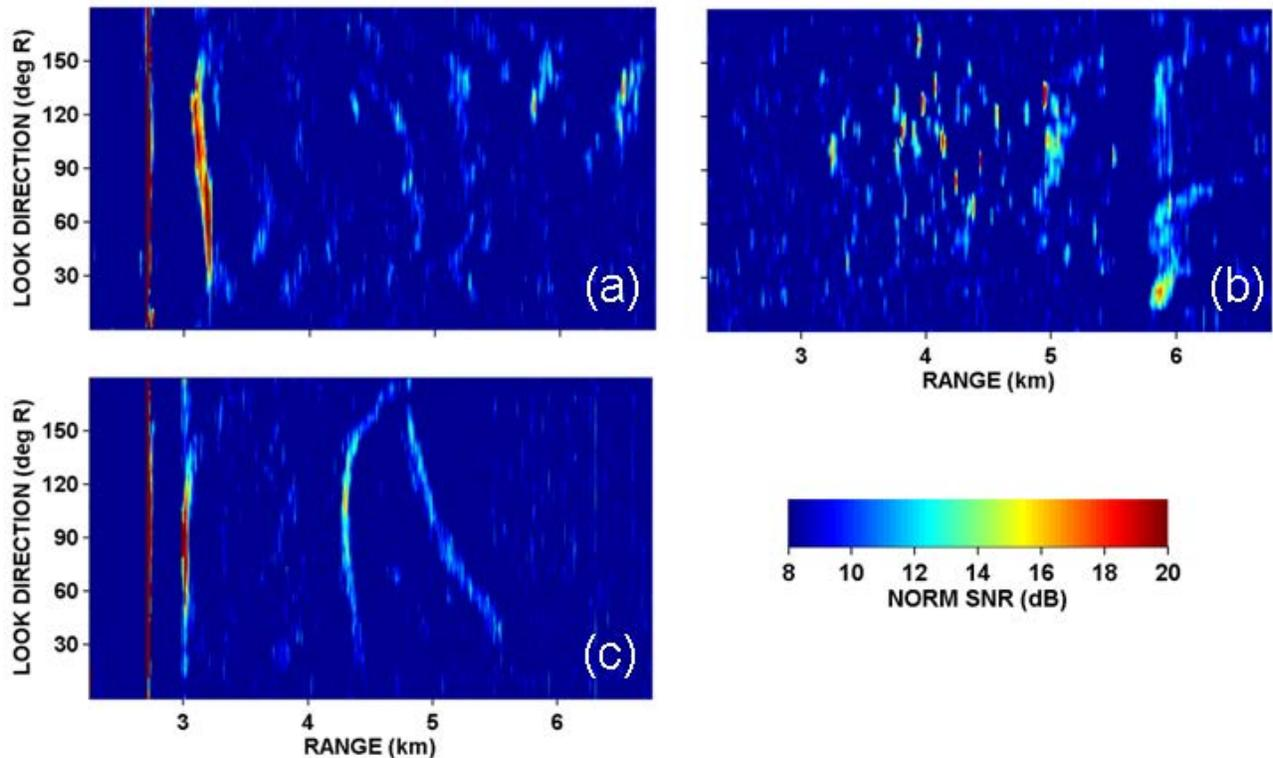
**Fig.5. Representative clutter (normalized match-filter) data collected in three geographic areas: (a) Astoria Canyon ( $\sim 46.1^\circ\text{N}$ ; box 1, Fig. 1); (b) north of Heceta Bank ( $\sim 44.5^\circ\text{N}$ ; box 4, Fig. 1); and (c) south of Heceta Bank ( $\sim 43.4^\circ\text{N}$ ; box 5, Fig. 1). (The strong echoes at  $\sim 2.7$  and  $3.1$  s in (a) and (c) are from the direct blast and seafloor respectively.)**
