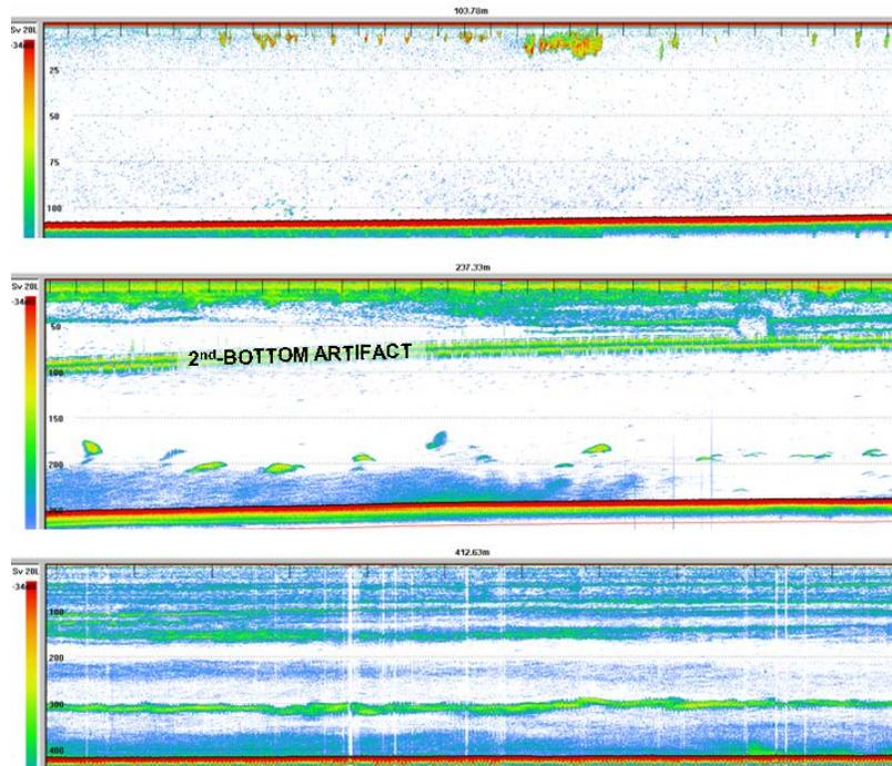
**Fig.4. Experimental 18-kHz Simrad observations (30-min traces): (top) in shore (~45.8°N; green circle, Fig. 3-left) at night; (middle) west of Arch Cape (~45.9°N' box 2, Fig. 1) in the late afternoon; and (bottom) south of Heceta Bank (~43.4°N; box 5, Fig. 1) during the day. (Note the different depth scales)**
