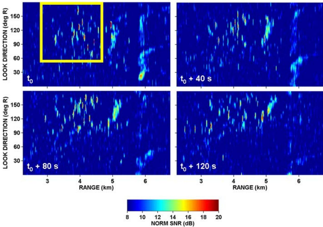
**Fig.6. Clutter (normalized match-filter) data from four successive pings (40 s apart) collected north of Heceta Bank (~44.5°N; box 4, Fig. 1).**
