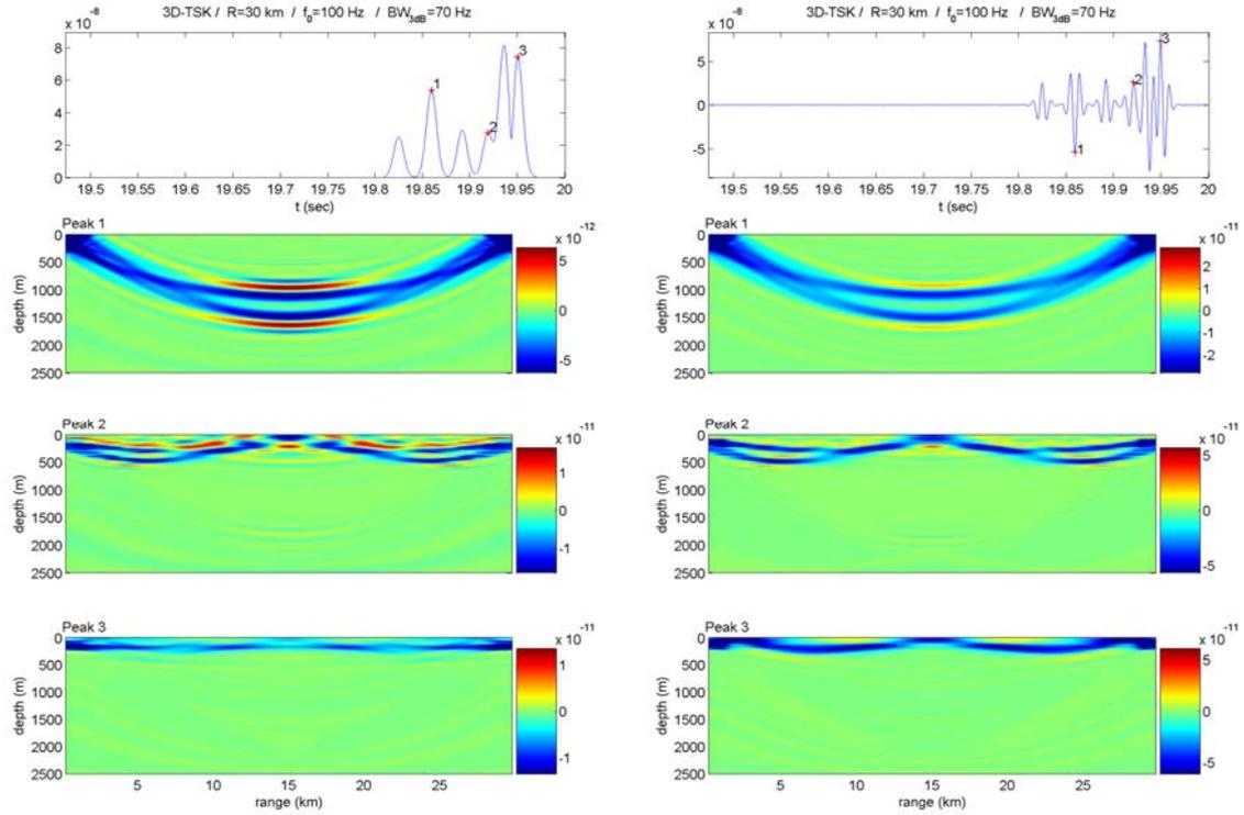
**Fig. 2. 3D propagation results at 30 km range. Left: Arrival pattern (top) and sensitivity kernels (lower) for peak arrival times of marked peaks. Right: Acoustic pressure (top) and sensitivity kernels (lower) for phase arrival times of marked peaks.**
