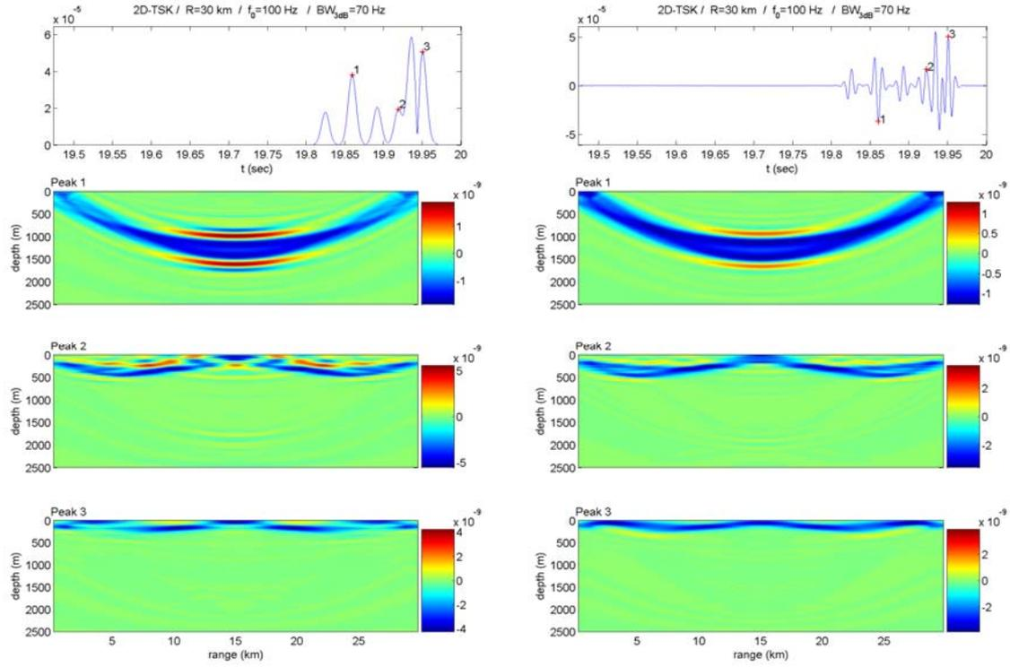
**Fig. 3. 2D propagation results at 30 km range. Left: Arrival pattern (top) and sensitivity kernels (lower) for peak arrival times of marked peaks. Right: Acoustic pressure (top) and sensitivity kernels (lower) for phase arrival times of marked peaks.**
