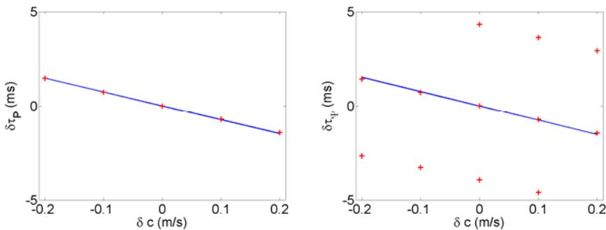
**Fig. 6: Actual (+) and predicted (line) travel-time perturbations for peak (left) and phase (right) arrival times for arrival 3 and sound-speed perturbations about 150 m depth**
