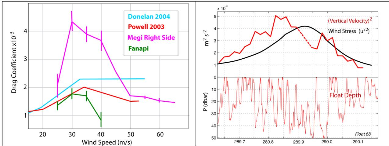
**Figure 1.** Left) Drag coefficient computed from upper ocean momentum budget using data from EM-APEX floats deployed in T. Fanapi (green) and T. Megi (magenta) compared to laboratory (cyan) and dropsonde (red) estimates. Megi shows very large drag at 30-40 m/s. Right) Vertical kinetic energy (top) computed from Lagrangian float data (bottom) from T. Megi leads wind stress computed from aircraft wind speed (black) by several hours.
