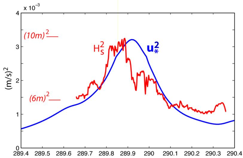
**Figure 3.** Significant wave height squared (red) and wind stress (blue) on the right side of Typhoon Megi computed from Lagrangian float data. The peak waves occur before peak winds. This may explain the very high drag coefficients found near the peak waves.
