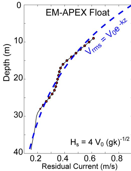
Figure 1. Exponential increase in high-frequency velocity measured on each EM-APEX profile is used to compute the significant wave height  $H_s$  and wavenumber as shown in this example. Wave frequency is computed from the dispersion relationship  $\sigma = (gk)^{1/2}$ .
