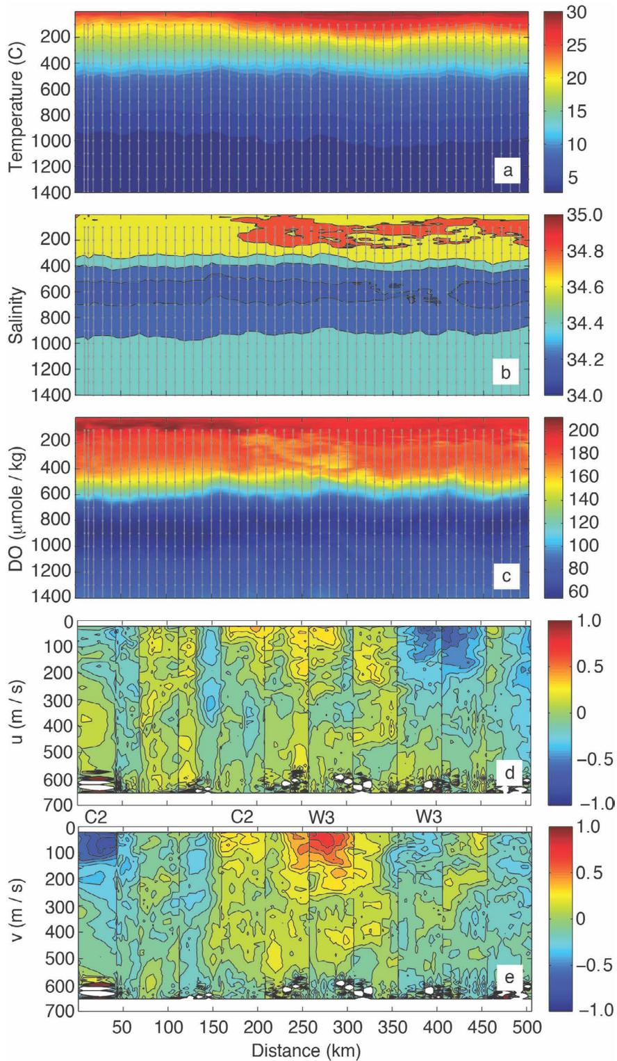
**Figure 2.** CTD and hull-mounted ADCP velocity sections across eddies C2 and W3. The section location is shown in Figure 1. From top to bottom, the sections display a) temperature, b) salinity, c) dissolved oxygen, d) zonal velocity, and e) meridional velocity. The velocity data are hourly averages from the 75 kHz ADCP.
