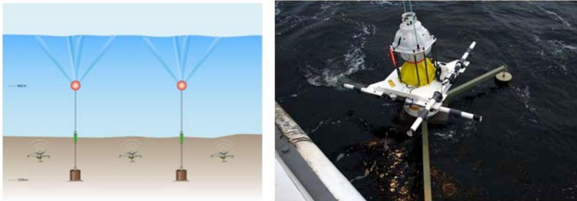
*Fig. 7: Illustration of HPIES (right panel) deployed in relation to R-C Lien's ADCP mooring array (left panel). The HPIES consists of the URI CPIES on top. This unit measures travel time of acoustic pulses to and back from the surface and bottom pressure. The HEF unit is in the yellow hard hat with electrode arms and water switches on the white plastic platform.*
