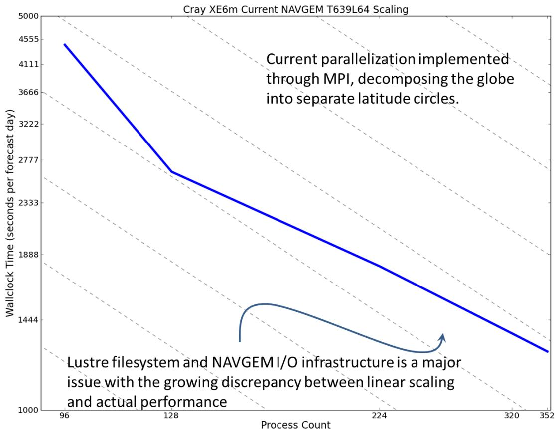
**Figure 1 – Plot showing seconds per forecast day wallclock time for a T639L64 (~21 km at the equator) NAVGEM integration. Dashed slanted lines show “perfect” scaling (i.e. double the number of processors, cut wallclock time in half). The growing discrepancy between ideal scaling and actual scaling includes contributions from computational limitations (e.g. the spherical harmonic transforms) as well as system limitations, primarily input/output.**
