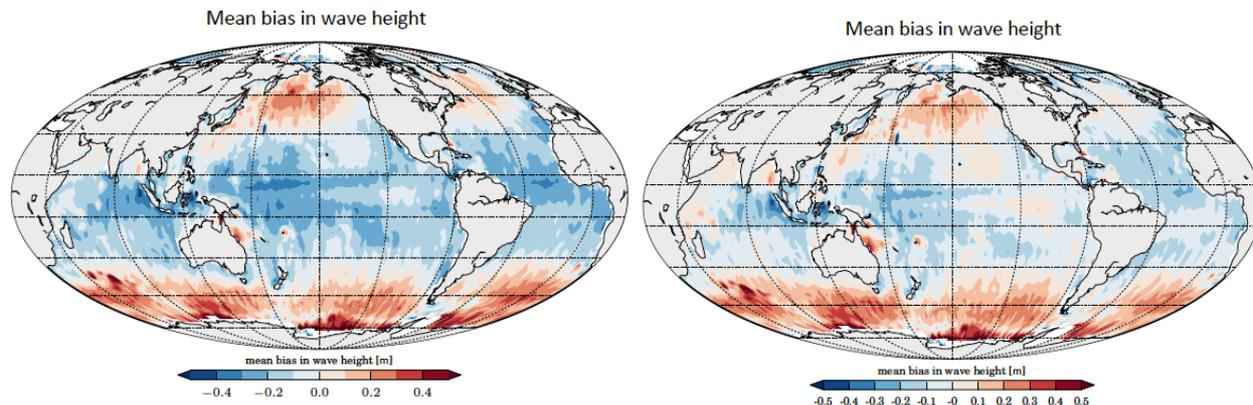
Figure 1. Bias of the global 2013 WAVEWATCH-III hindcast with respect to CRYOSAT2 observations. Scale is in units of meters at the bottom. (left) constant decay coefficient; (right) steepness depended decay coefficient for swell.
