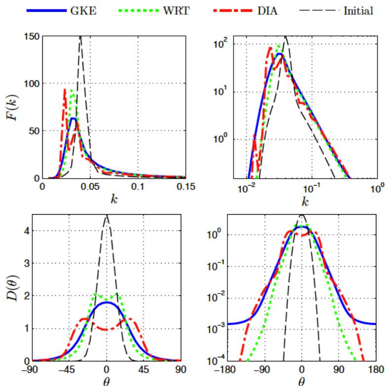
Figure 2. Evolution of JONSWAP-like spectrum with  $\cos^n$  directional distribution ( $n=32$ , JONSWAP's  $\alpha = 3.7 \cdot 10^{-3}$  and  $\gamma=20$ ). Dashed line is the initial spectrum, other spectra are shown after 1000 period of nonlinear evolution due to GKE (solid blue), WRT (dotted green), DIA (dash-dotted red). Top panels are for the wavenumber spectrum and bottom for the directional spread; left panels are linear and right panels logarithmic
