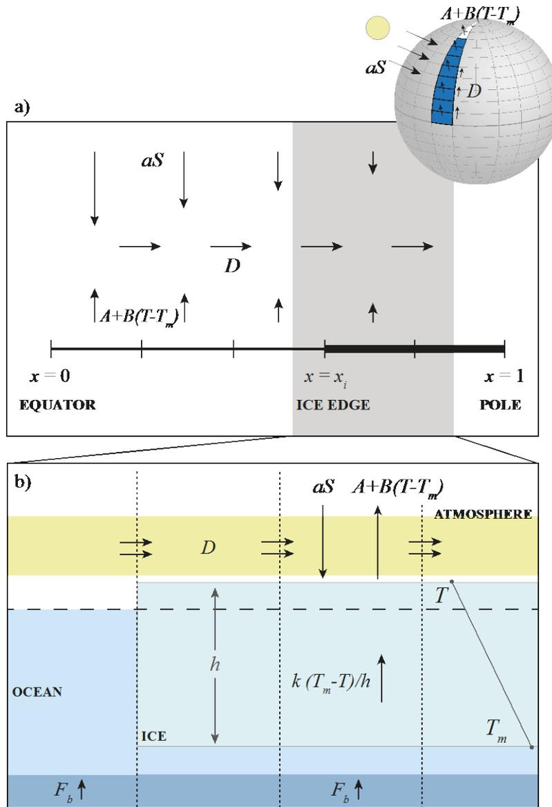
**Figure 1: Schematic of the global sea ice and climate model developed under this project. Globe inset: Illustration of the model domain, a zonally-averaged aquaplanet. (a) Energy fluxes in the model atmosphere in the full model domain. (b) Energy fluxes in the model atmosphere, sea ice, and ocean in a subset of the model domain near the ice edge.**
