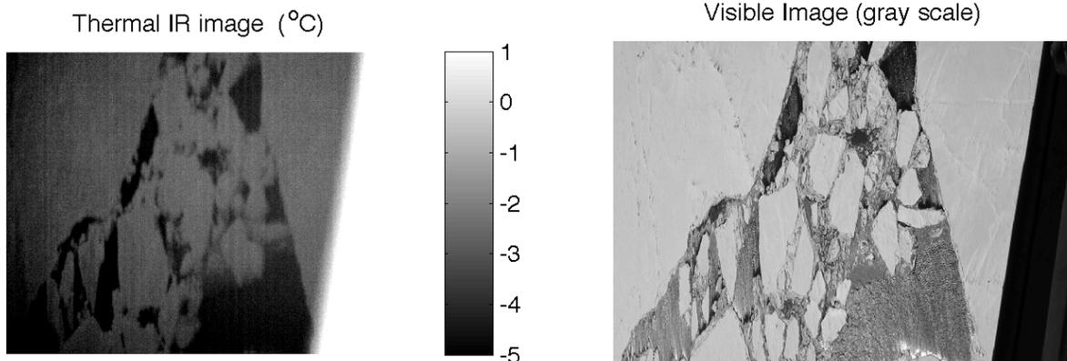
**Figure 2. (left) thermal IR image (right) visual band image from 300' altitude at 73°N taken on 17 June 2014. The thermal image shows that the water surface is approximately 2-3C cooler than the ice surface. The triangular sections on the right side of each image are where the side of the plane is visible (warm in IR and dark in visible).**
