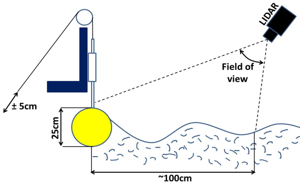
**Figure 2. Lab experiment setup. A solid ball (bowling ball, yellow) with a diameter of 25.0 cm was forced to bounce at the water surface in a 2.0 m deep cylindrical tank with a 3.3 m diameter. The Reigl VZ1000 Lidar was used to capture the wave surface as well as the ball location.**
