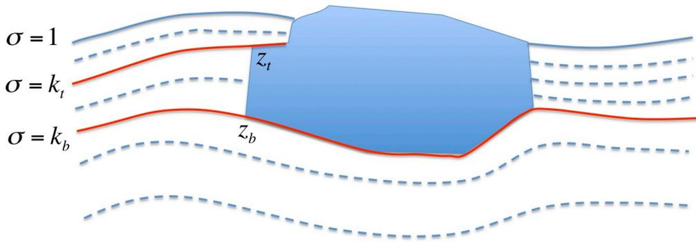
**Figure 1. Flexible sigma-coordinate for modeling wave-ice floe interaction.  $k_t$  and  $k_b$  represent sigma levels and  $z_t$  and  $z_b$  represent  $z$  values of vertical coordinate at the top and bottom of an object, respectively.**
