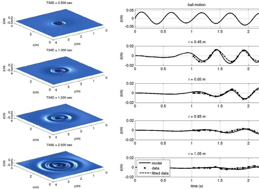
**Figure 3. Model results of the bouncing-ball experiment conducted at NRL, Stennis Space Center. (Left) Snapshots of wave surface modeled by NHWAVE at time=0.5,1.0,1.5 and 2.5sec. (Right) comparison of surface elevation between model and data (crosses: data, dashed lines: data fitted lines, solid lines: model results).**
