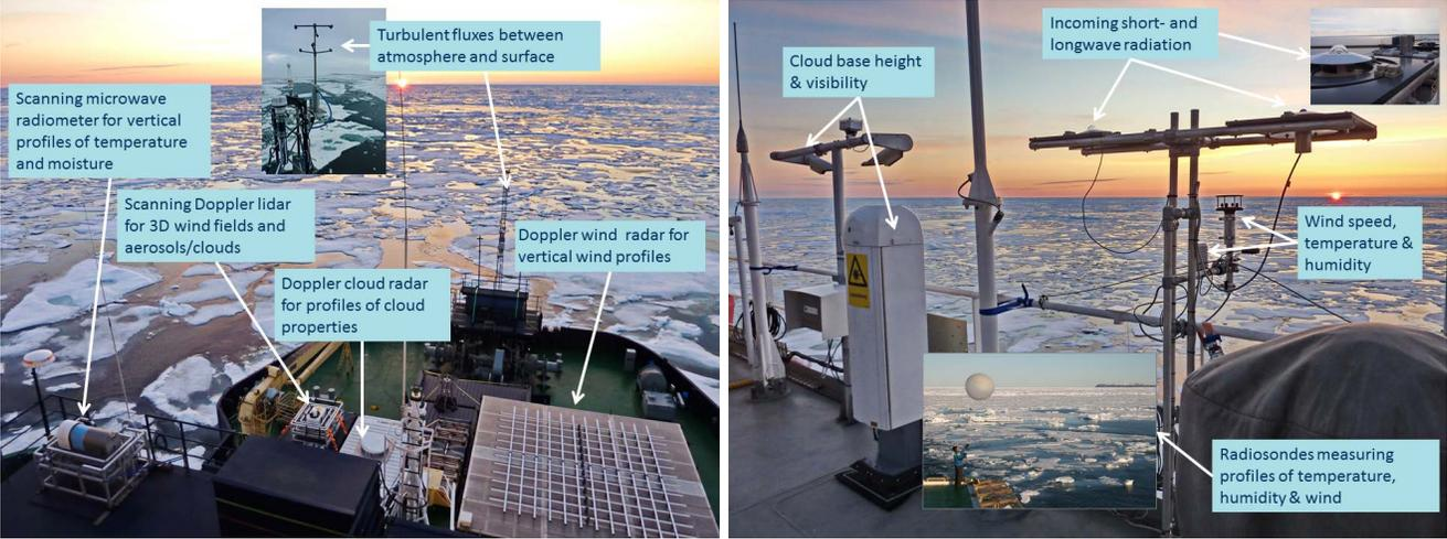
**Figure 1.** Photo overview of some instruments deployed on the Oden for ACSE showing (left) remote sensing instruments and bow mast from the 7<sup>th</sup> top deck, and (right) instruments on the 7<sup>th</sup> deck and sounding release on the helideck of Oden.
