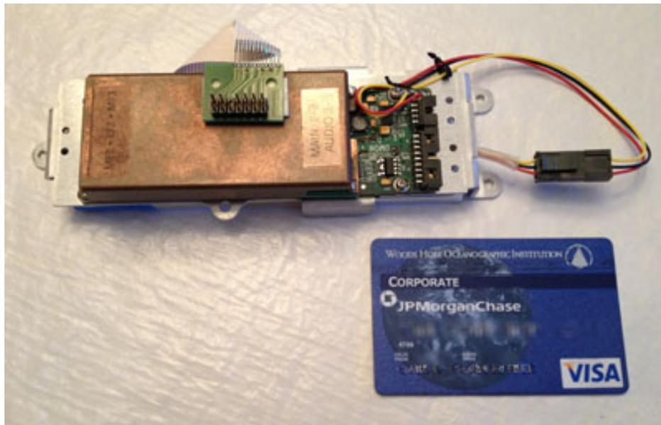
***Figure 1. Digital acoustic monitoring (DMON) instrument.
