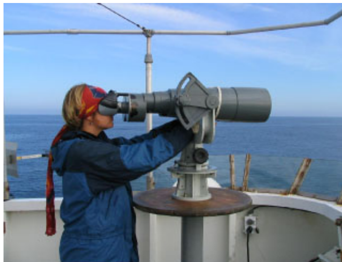
Figure 1. Fujinon 25×150 MTM “big-eye” binoculars being used at sea.
