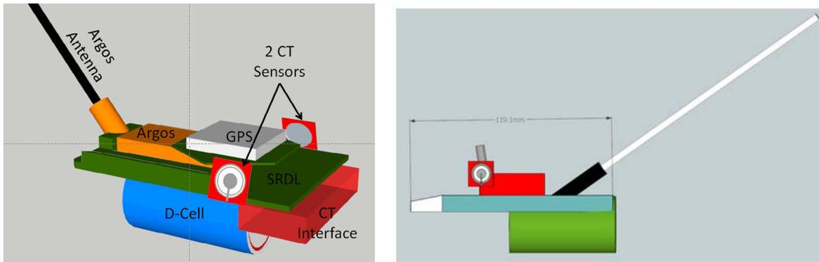
**Figure 2: Two design studies for electrode based CTD tags for non-rigid attachment. Instrument on the left has two CT sensors and a GPS receiver, while the right one has one CT sensor. The epoxy body is not shown.**
