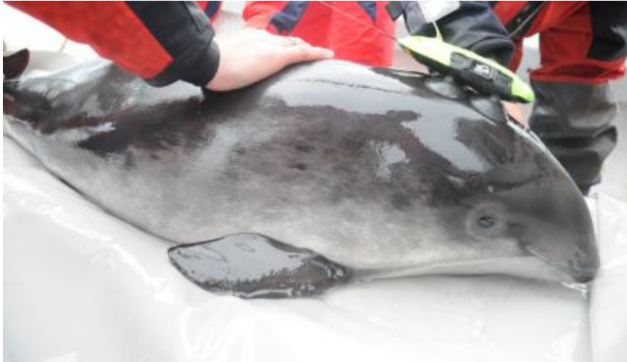
Figure 2: Prototype high frequency smart tag attached to a harbour porpoise in Denmark. This short-term version of the tag can record and process data for two days at the high sampling rate needed for porpoises. Operation for up to 4 days would be obtained on lower frequency cetaceans such as beaked whales.
