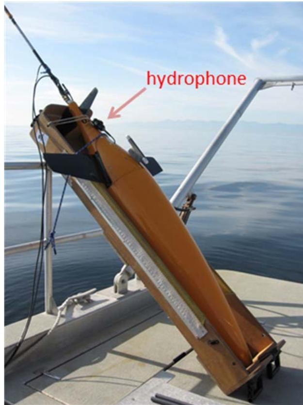
*Fig. 1. A Seaglider™ equipped for passive acoustics.*
