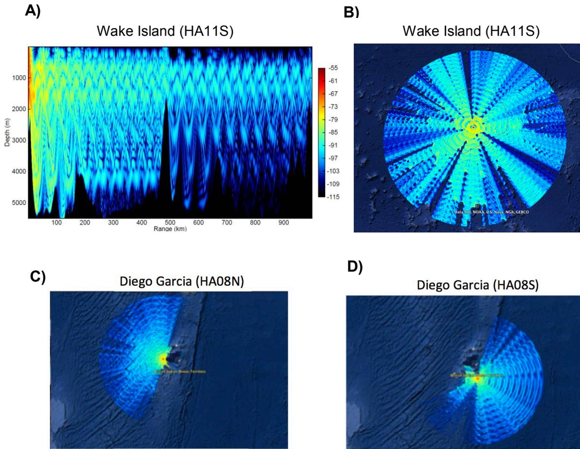
**Figure 1.** *A) Receiver modeling TL output from the Peregrine PE model at CTBTO location at H11 S1 in the Pacific Ocean at Wake Island during the winter season (20 Hz, 1000 km range). TL is shown as a function of depth and range at 280° bearing. B) TL receiver output from the Peregrine PE model as a function of range around HA11 S1 at Wake Island. C) TL receiver output from the Peregrine PE model as a function of range around HA08 N1 and (D)HA08 S2 in the Indian Ocean at Diego Garcia.*
