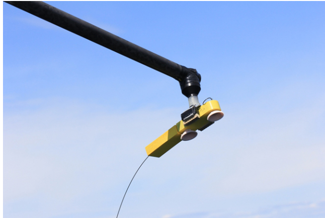
Figure 1. Tag mounted on pole using a modified DTAG “robot”
