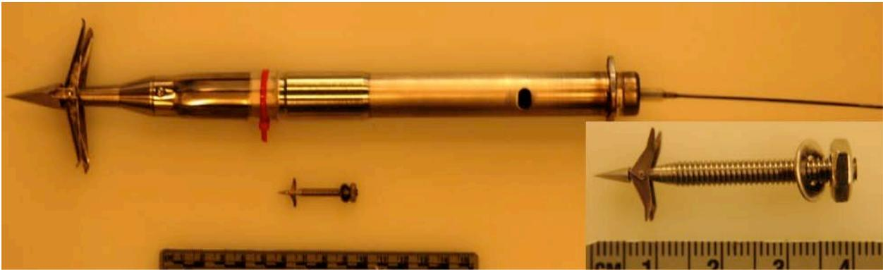
**Fig. 3 – Large whale transdermal satellite tag and 1/7<sup>th</sup> scaled dolphin dummy tag. Inset shows dummy at a larger scale. Scales in cm.**
