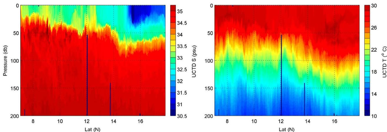
**Figure 2: Salinity (left) and temperature (right) from the Underway CTD system during the December 2013 cruise on the RV *Roger Revelle*. The data are from a straight transect referred to as “section B” in Lucas et al. (2014), extending from about 8°N, 85°E (near Sri Lanka) to 18°N, 89°E (near the northernmost point of international waters in the Bay of Bengal).**
