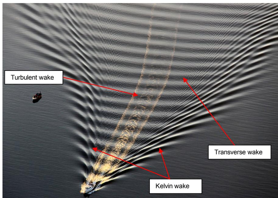
***Figure 1: Optical image of a ship wake showing the different wave patterns produced by a ship. The bow wave is oriented at the Mach angle of  $19^{\circ} 28'$  and the transverse wake are circular waves emanating from the ship's stern. © 2009 Chris Goldberg used by permission.***
