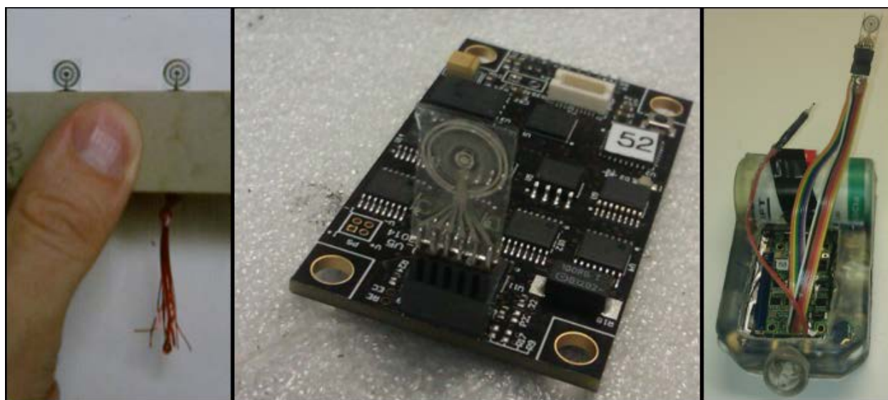
Figure 1: Two CT sensors (left), a single CT sensor including interface board (middle) and a CT package integrated into a SRDL (right) are shown.
