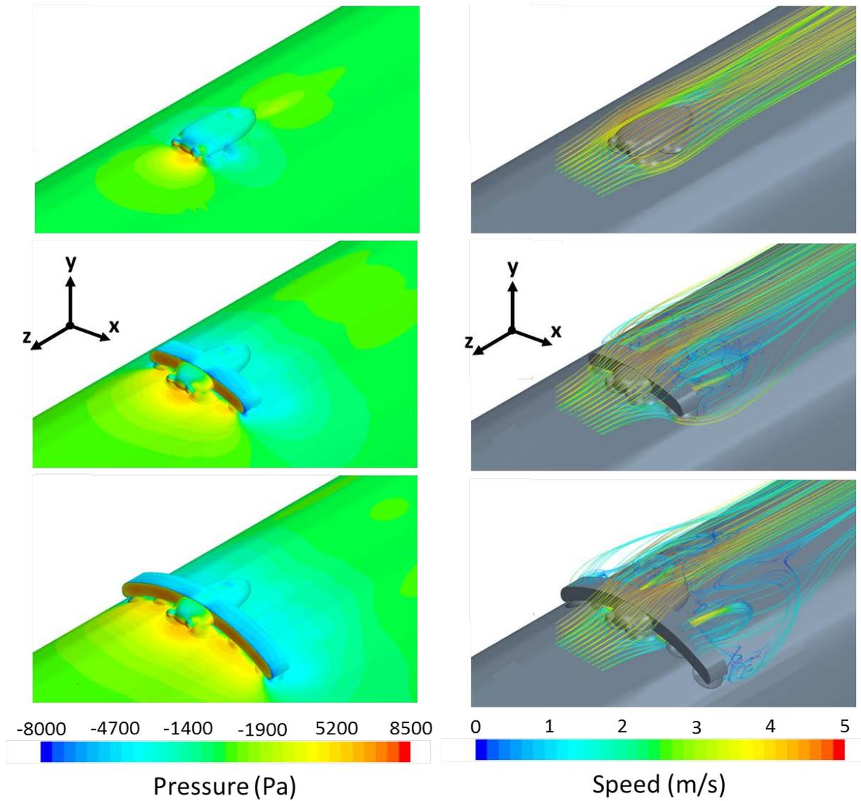
**Figure 1.** CFD simulation results of the DTAG (top) and additional drag elements used to increase the frontal area by factors of two (tag+2, middle) and four (tag+4, bottom) in 4 m/s inline flow. Pressure is mapped to the surface geometry and is shown on the left, and stream lines with the corresponding fluid speed are shown on the right.
