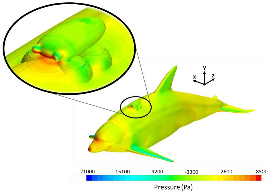
***Figure 2. CFD simulation results of the DTAG and representative dolphin geometry in 4 m/s inline flow. Pressure is mapped to the surface geometry with high pressure (slow moving fluid) shown in red and low pressure (fast moving fluid) colored in blues and greens.***
