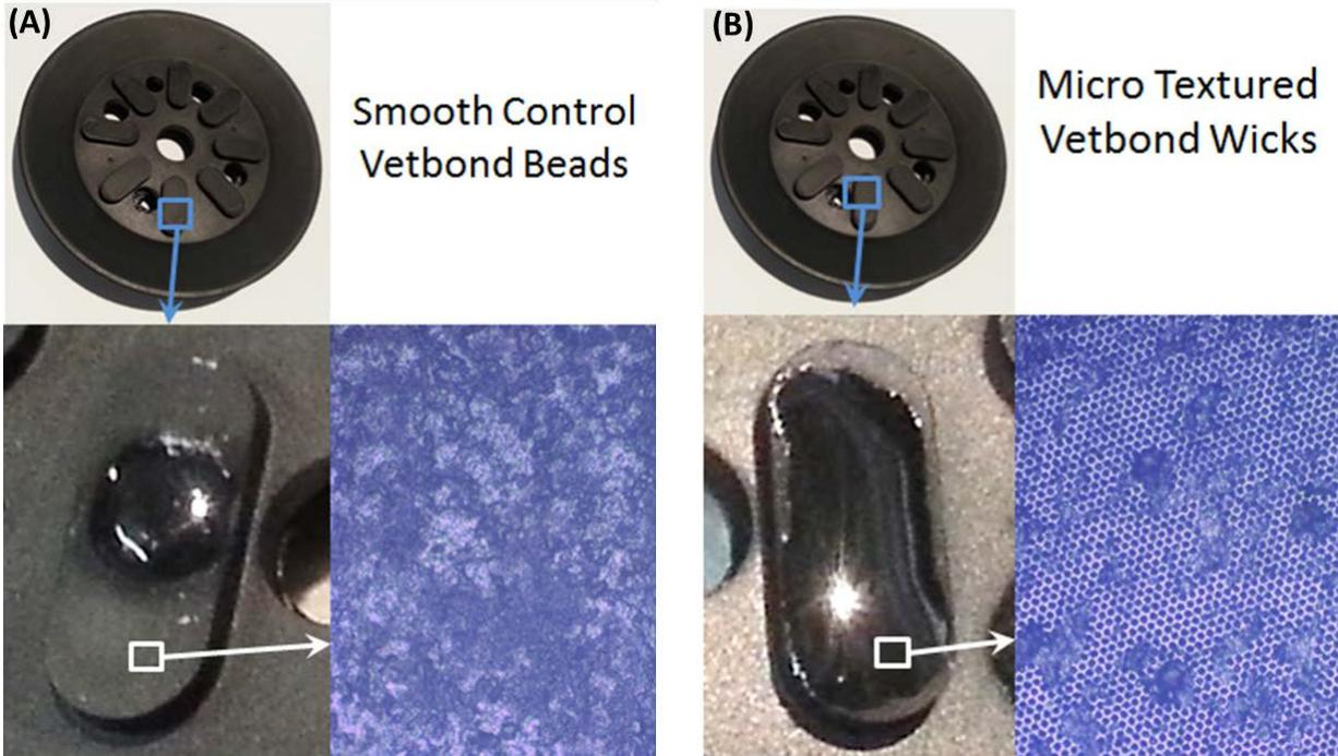
**Figure 3.** The proposed hybrid suction cup shown (A) without micro-texturing and (B) with micro-texturing. The improved wetting properties imparted by the texturing are shown in the figure details. A droplet of glue placed on the untextured surface has does not spread (bottom left), while the droplet on the textured surface spreads to the edges of the feature (bottom right).
