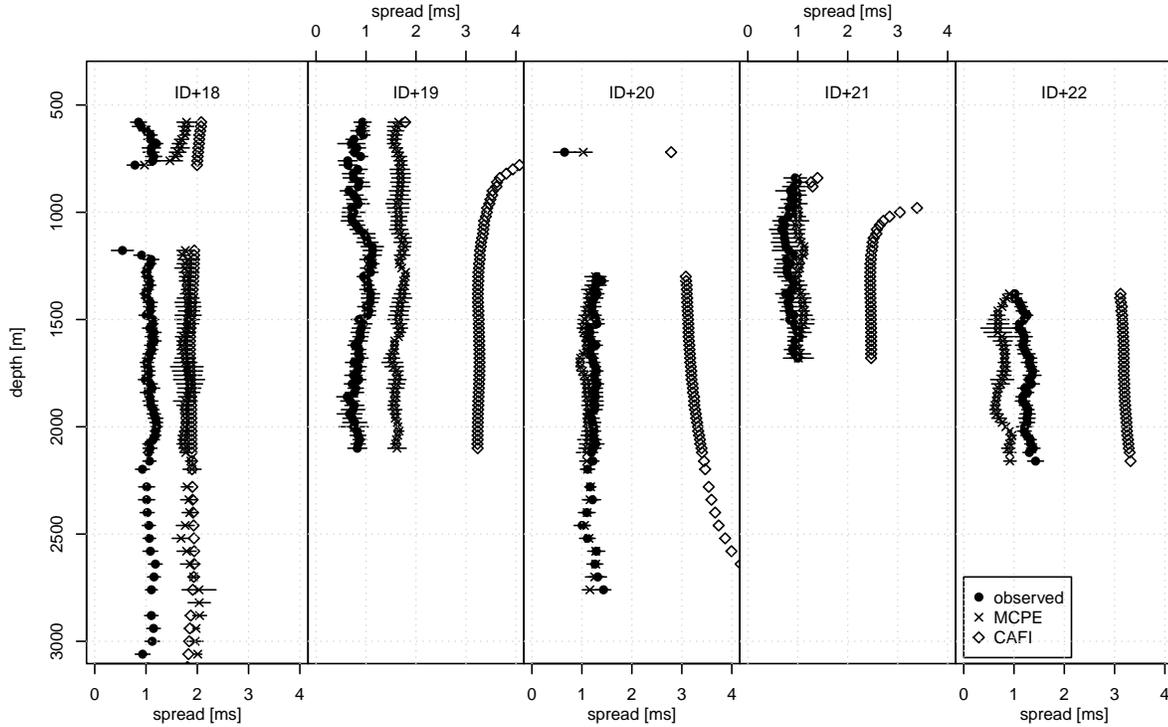
**Figure 9: Pulse spreads measured for ray IDs +18, +19, +20, +21 and +22 for the MP200/TR1446 red signal. Parametric (Gaussian fit) method. Error bars are  $\pm$  two standard errors.**
