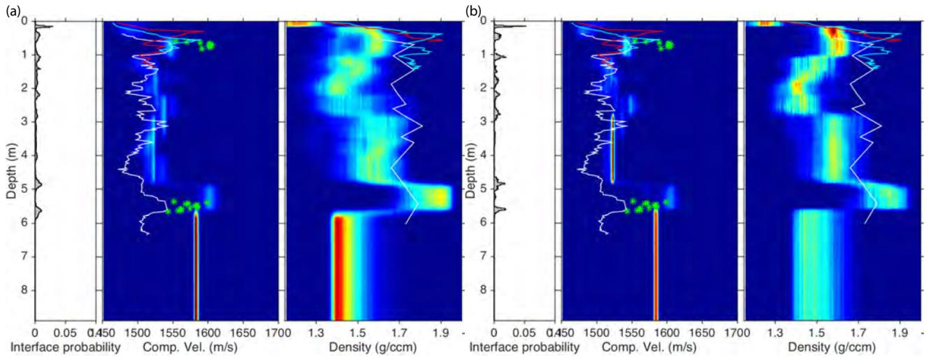
**Figure 4: Comparison of geoaoustic profiles for sound velocity and density for two inversions of the same data (a) without and (b) with the ENOS prior. Several core measurements are also shown for comparison.**
