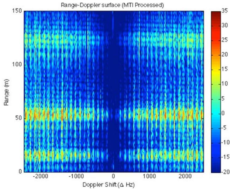
**Figure 3:** Measured spectrum of received signal after clutter filtering, here shown as a radar delay-Doppler surface. The clutter filtering is a simple MTI filter. The spectrum of each node is clearly seen at a distance of approximately 15m, 50m, and 130m.
