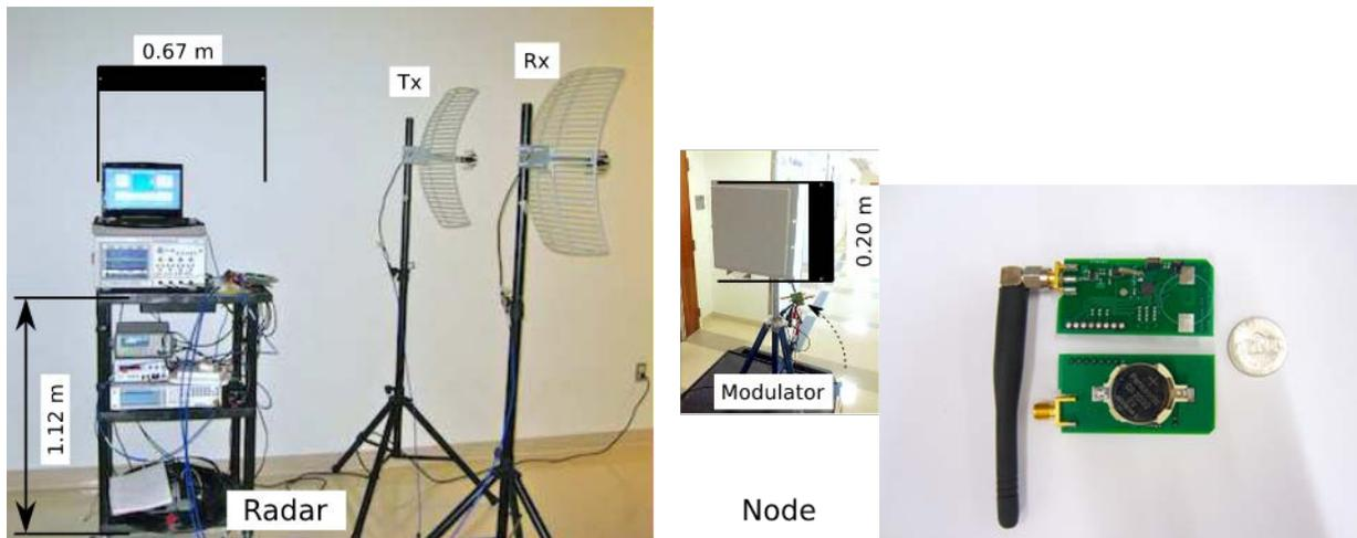
**Figure 2: Experimental setup. The radar hardware is shown on the left, including waveform generator and transmit and receive high-gain antennas. The node hardware is shown on the right including a closeup of the node board with a US nickel for scale reference.**
