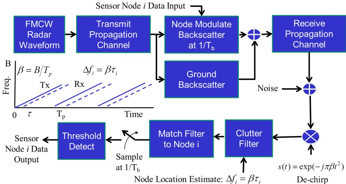
**Figure 1: Simplified Signal Processing Chain for PEEMS**
