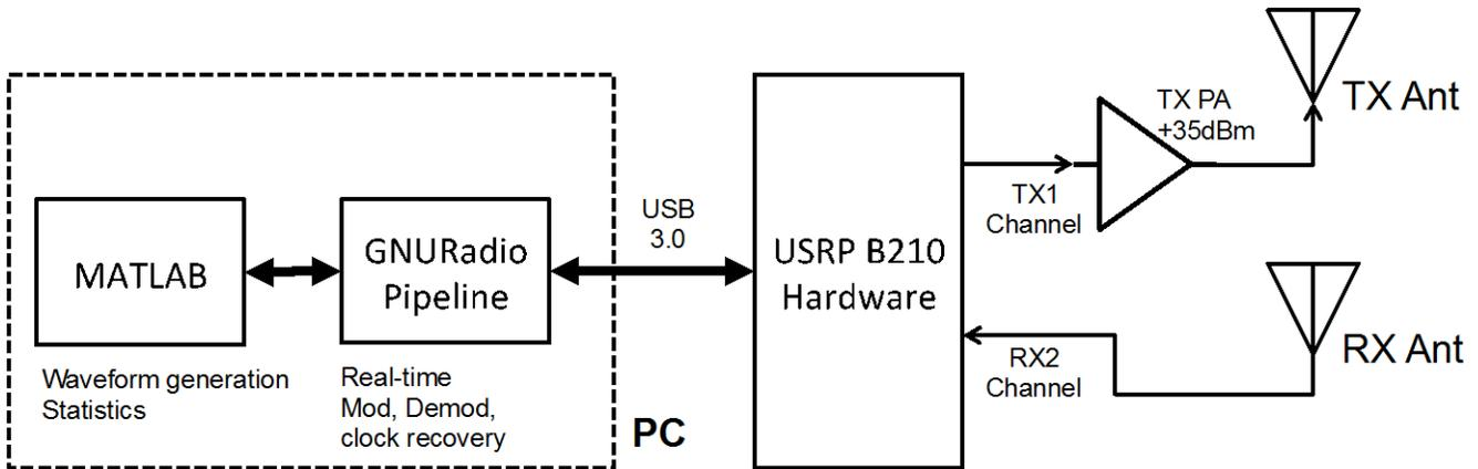
**Figure 5: Block diagram of the software-defined radar hardware**
