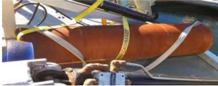
Figure C: Open-ended steel pipe used as a target during the Massachusetts Bay experiment, sitting on the deck of the R/V *Resolution*. The pipe is 1.5 feet in diameter and 5 feet long.
