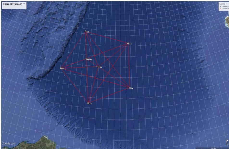
**Fig. 1. The 2016–2017 CANAPE Experiment will consist of six tomographic transceivers ( $T_1, T_2, \dots, T_6$ ) and a DVLA receiver located approximately at the intersection of the  $T_1$ - $T_4$  and  $T_2$ - $T_5$  paths. The array radius as shown is 200 km.**
