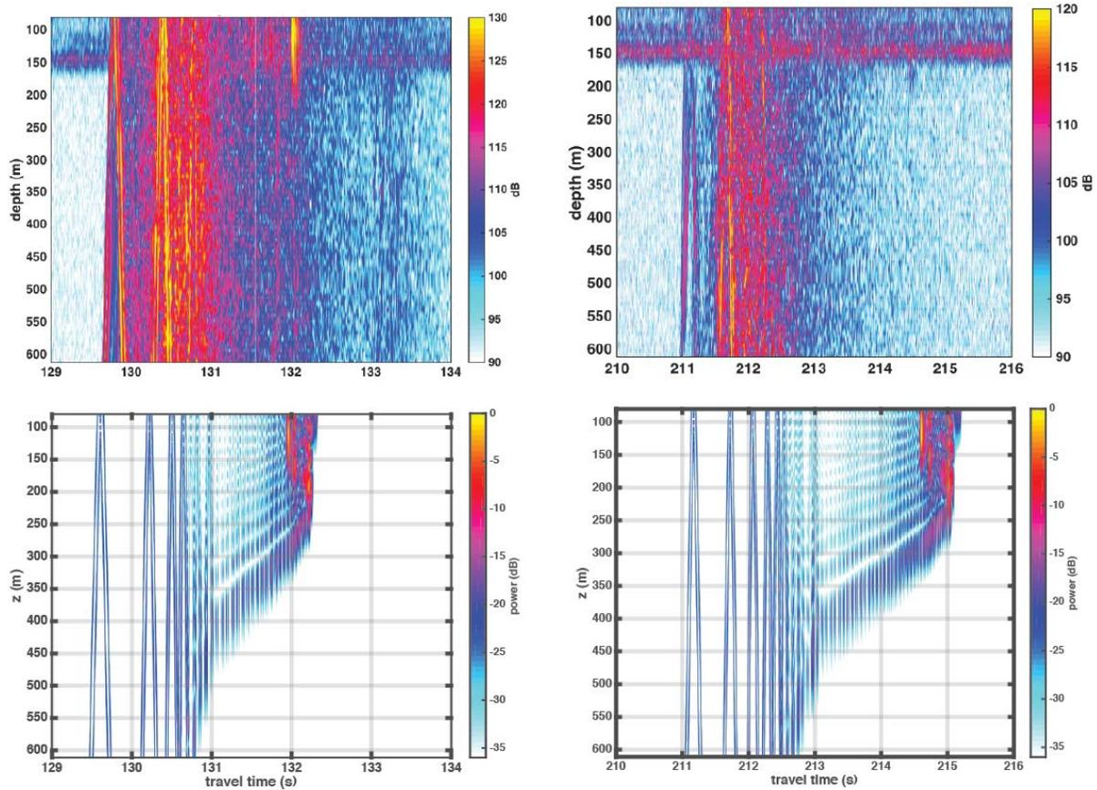
**Fig. 3. Measured (top) and predicted (bottom) arrival patterns on the DVLA for HLF-5 transmissions on year day 222 at 1500 UTC at about 190 km range (left) and on year day 224 at 1000 UTC at about 309 km range (right).**
