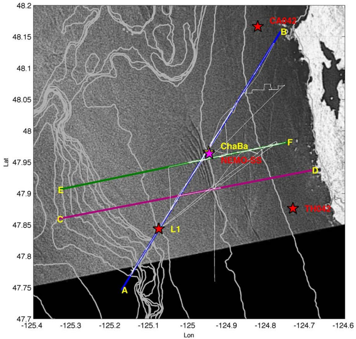
**Figure 1:** High Resolution bathymetry contours of the study region, mooring locations and survey lines. Synthetic aperture radar (SAR) imagery showing the wave crests traveling onshore is overlaid. Contours are every 50 m until 500 m, and then every 200 m after that.
