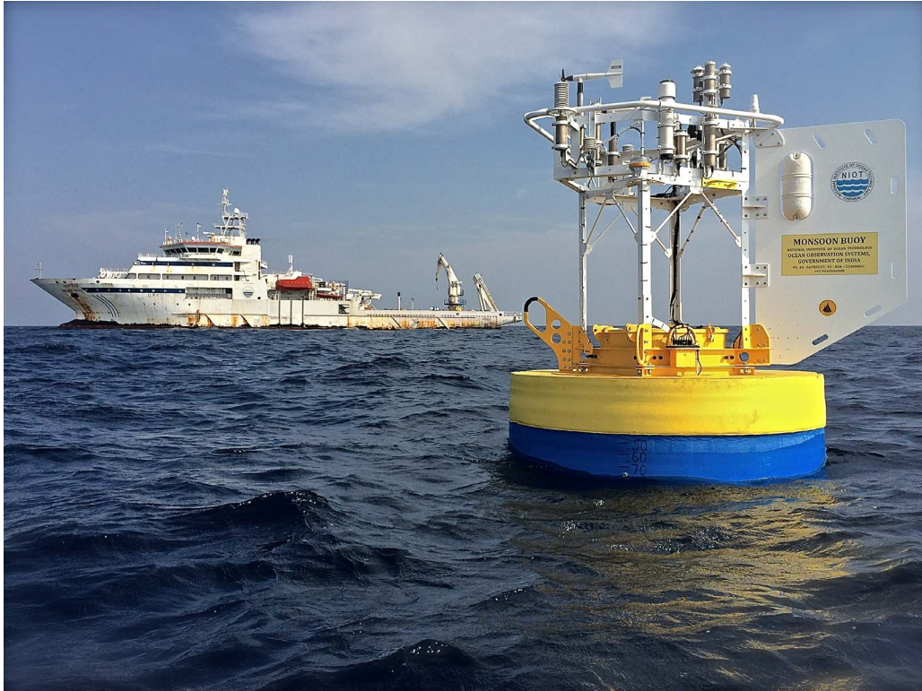
Figure 1: The surface buoy of the surface mooring deployed in December 2014 in the northern Bay of Bengal is shown with the ORV Sagar Nidhi in the background.
