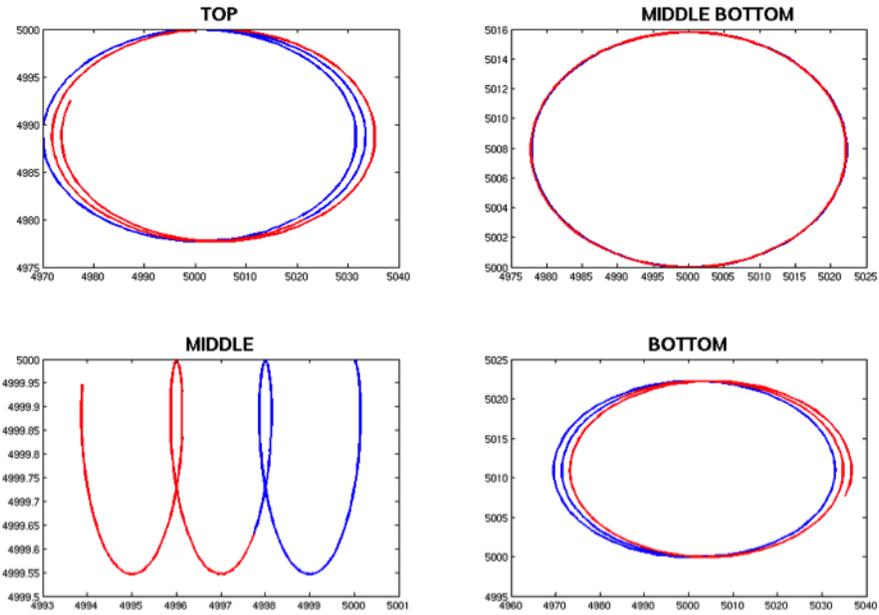
**Figure 2: Trajectories of Lagrangian particles initially placed at different vertical positions in a mode-1 internal-wave field. Early-time displacements are in blue, later-time displacements are in red. Axis units are meters and mean stratification is linear.**
