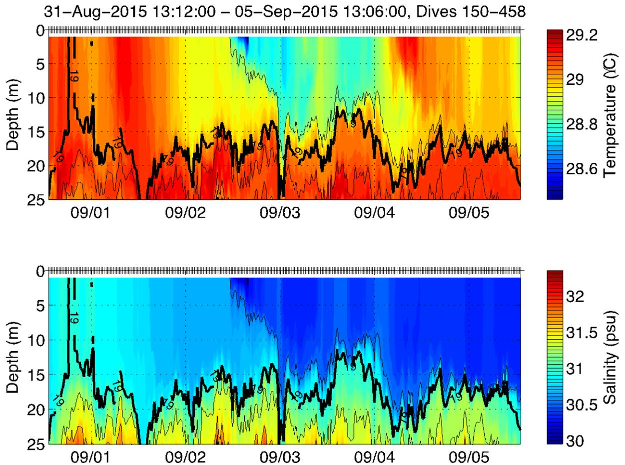
**Figure 2.** Temperature and salinity (color shading) and potential density (black contours) as functions of time and depth from a prototype  $\chi$ SOLO in the Bay of Bengal. The upper 25 m are shown from a float that profiled over the upper 50 m. Time tick marks are at midnight GMT, near the time of sunrise at the float's location. Note the shallow cold, fresh layer formed by rainfall on 2 September. The diurnal cycle is apparent in temperature.
