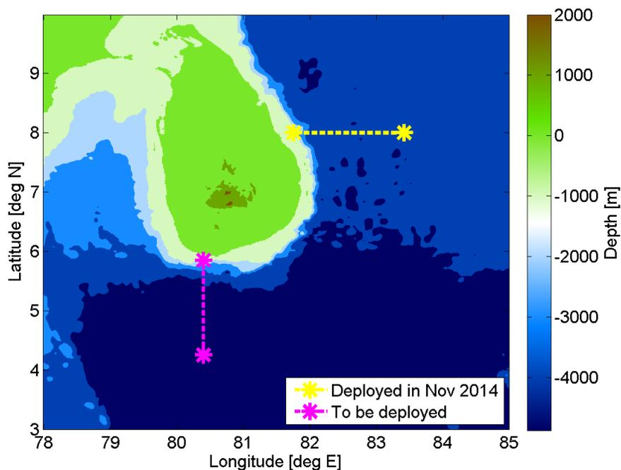
**Figure 1:** Map of Sri Lanka with the eastern and southern sections highlighted. The eastern section follows roughly  $8^{\circ}\text{N}$ , while the southern section is on  $80.4^{\circ}\text{E}$ . Deployment locations for the PIES are indicated as stars (actual on the eastern section, planned on the southern section).
