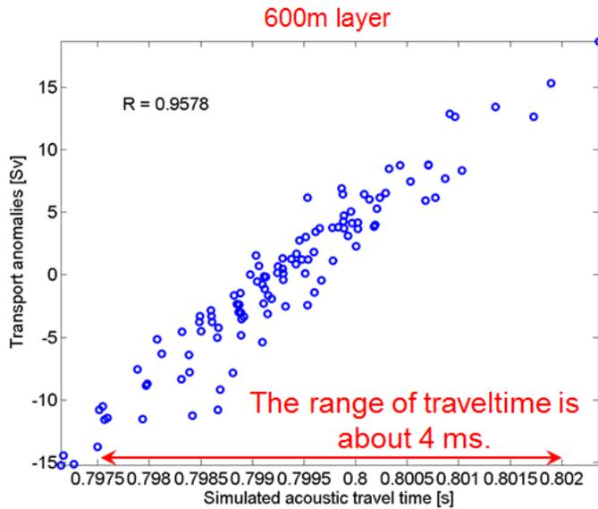
**Figure 4:** Simulations of PIES acoustic traveltime (x-axis) for pairs of CTD data, which can be translated into geostrophic transport relative to the lower depth of the CTD profiles (y-axis). The signal for a 600m deep PIES is about 4ms, which is well measurable, and corresponds to the +/- 10Sv already expected from altimetry data.
