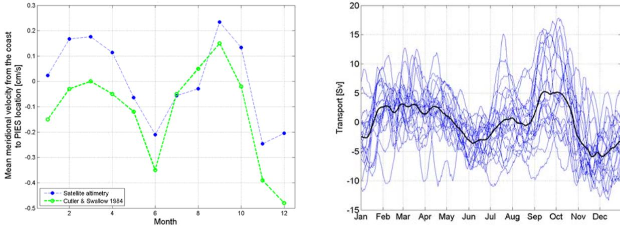
**Figure 3: Typical flow and transport variability of the boundary current on the eastern section out to the offshore PIES deployment location chosen. The panel shows the mean seasonal variability of the mean surface flow, and the right panel shows transport timeseries assuming a 100m scale depth for individual years.**
