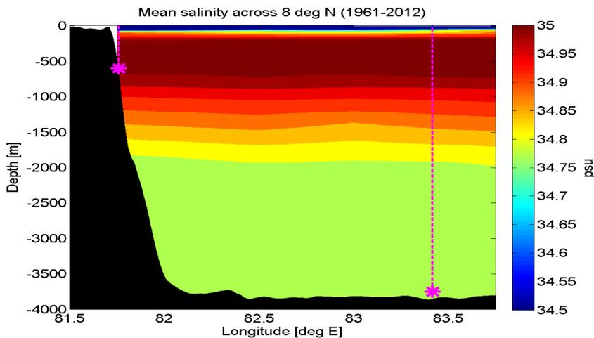
**Figure 5:** Section along 8°N showing the actual PIES deployment locations and depths, overlaid with a mean salinity field from historical CTD data. Note that the goal of the PIES measurements is measurement of the boundary current in the upper 100-200m, which dominated the vertical integral at both locations.
